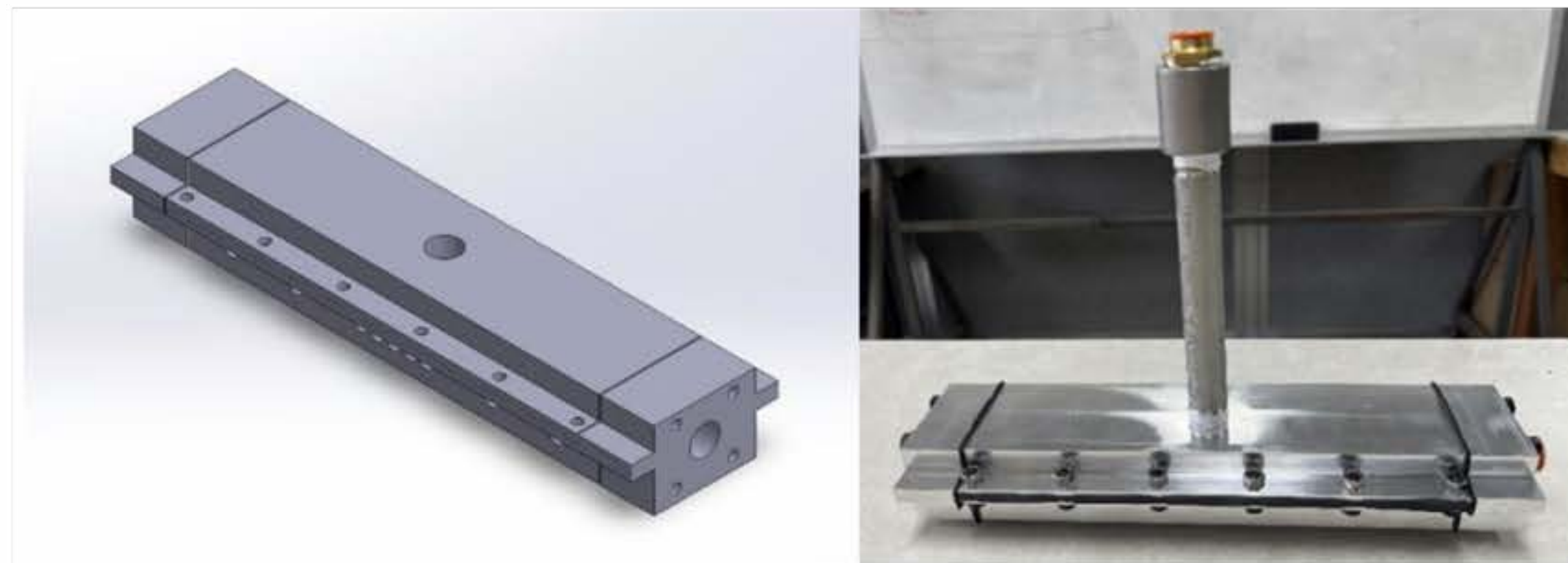
Fig. 1. CAD isometric view and manufactured setup of experimental test section.
